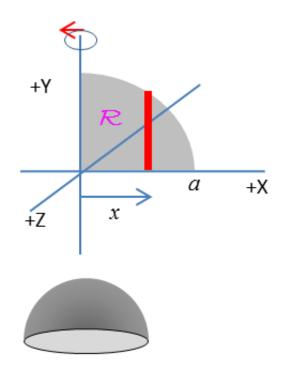
Volume of solid of revolution about the Y-axis using the cylindrical shell method is
