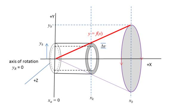
The area of each ring is  $A(x_k) = 2\pi y_k \Delta y$  (circumference x width) The volume of each the cylindrical shell is
