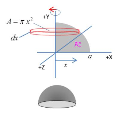
Volume of solid of revolution about the Y-axis using the **disk method** is
