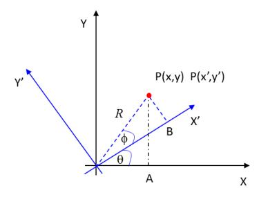
From the two right angle triangles shown in the figure, we can give the coordinates of the point P in Cartesian and polar coordinates for both sets of axes.
